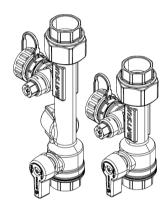
For quick isolation of the boiler DHW connections.
