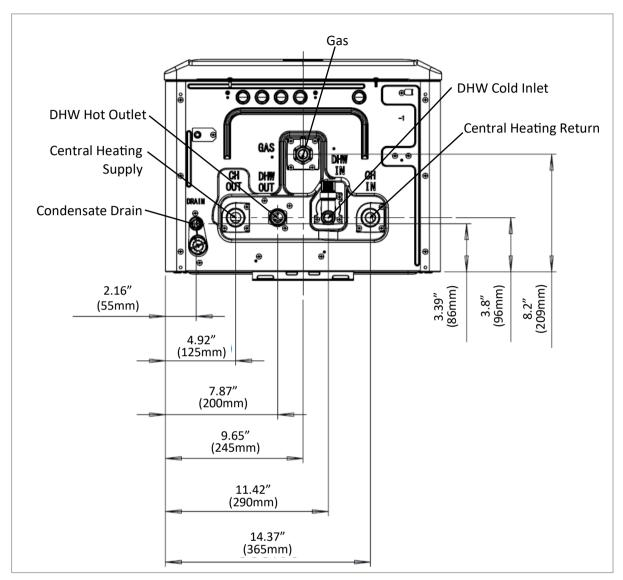
Figure 6: Supply Connections
